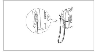
Pass the narrow end of the strap through the strap lug and pass the other end through the loop.
